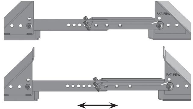
5. Place the clevis pin into the aligned holes, and then replace the cotter pin to secure it.
