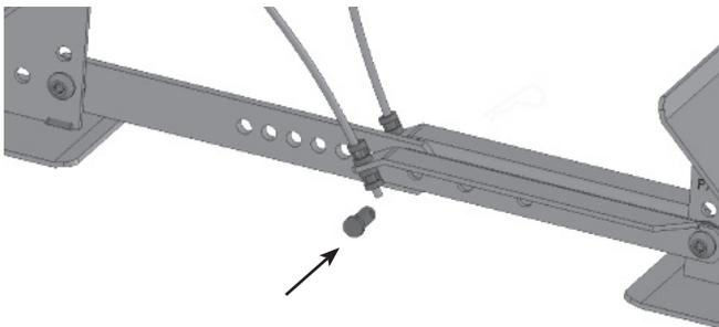
4. Remove the chock, and remove the clevis pin, then slide the arms apart until the next set of holes line up.
