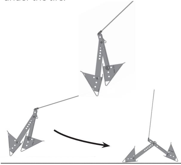
Others prefer to place the pin so that the arms hang at about the same length, and then step down on the tail ends of the wedges to force them open before sliding them between the wheels.
