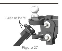
All nuts and bolts should be checked before each trip and tightened if necessary.
