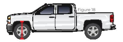
Measure from the ground to fender through the center-line of the axle.
