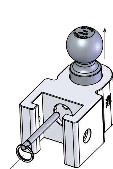
Figure 6 - Use the ring to remove the ball retaining pin.
