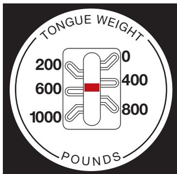
Figure 5 - Scale indicates a tongue weight of 500 lb.
