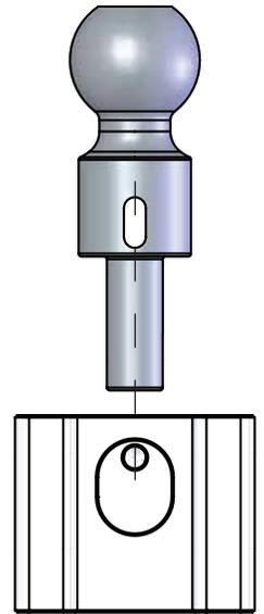
Figure 7 - Align the slot with the pin hole.
