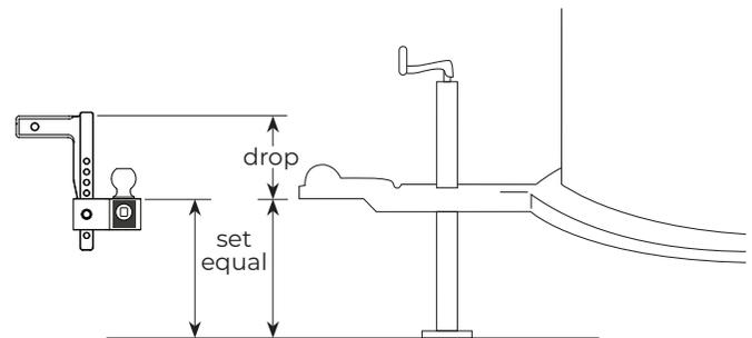
Figure 1 - With the trailer level, set the top of the ball holder at equal height to the bottom of the coupler socket.
