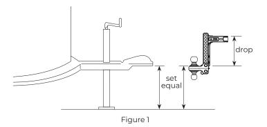
The top of the ball holder height should initially be set equal to the bottom of the coupler socket height with the trailer parallel to the ground, then adjusted upward to compensate for the distance it drops when the tongue weight is being carried. Rise or drop is measured from the top of the receiver opening to the top of the ball holder.
