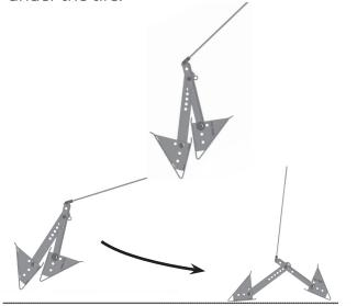
Others prefer to place the pin so that the arms hang at about the same length, and then step down on the tail ends of the wedges to force them open before sliding them between the wheels.
