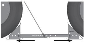
3. Slide the clevis pin into one of the holes in the arms to temporarily hold them in place. Don't insert the cotter pin yet.
