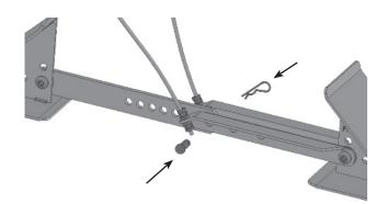
6. If you are not able to lengthen or shorten the chock to fit your axle spacing using the arm holes for adjustment, the bolts holding the ends of the adjustable arms can be moved. Use the included hex key (Allen wrench) and a socket wrench to move the bolts to either of the other two adjustment holes in the wedges.
