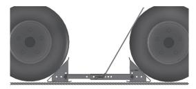
10. To remove the chocks, grasp the handle firmly in the middle and pull upward.
