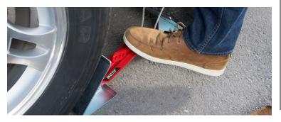
9. Lean the cable handle against the tire so that it is within easy reach when you want to remove the chocks.
