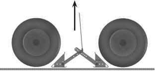
To lock the chock, step the chock into place tightly between the wheels. Place a padlock through one of the empty holes in the center of the arms, or through one of the lock holes in the wedges just above the scissor arms. Note: The lock is to be used as a theft deterrent. The lock will not guarantee the chocks can not be stolen.
