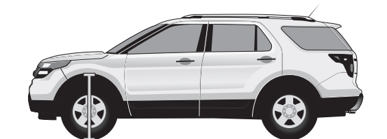
Figure 17 - Measure from the ground to fender through the center-line of the axle.
